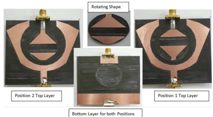
Fig. 10. The fabricated antenna prototype.
