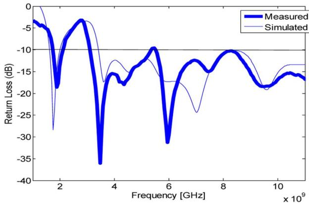
Fig. 11. The “sensing” antenna return loss.
