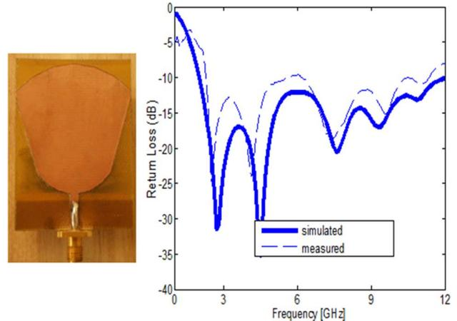
Fig. 1. The antenna structure and its return loss.
