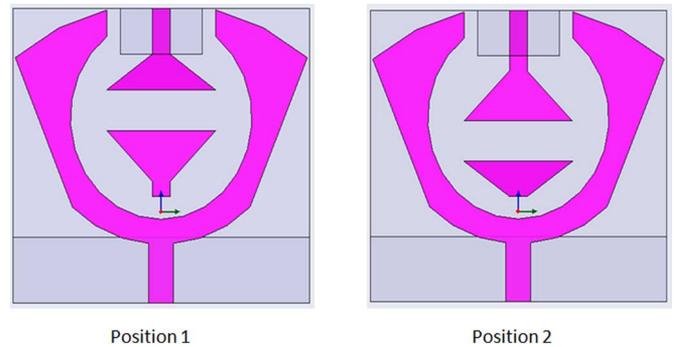
Fig. 9. The cognitive antenna structure.
