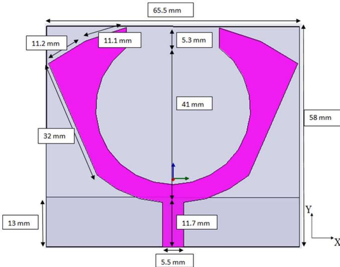
Fig. 2. The “sensing” antenna structure.
