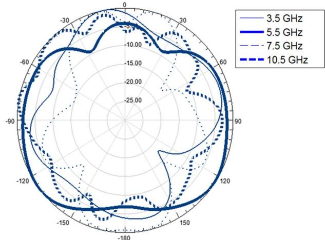
Fig. 14. The normalized antenna radiation pattern.
