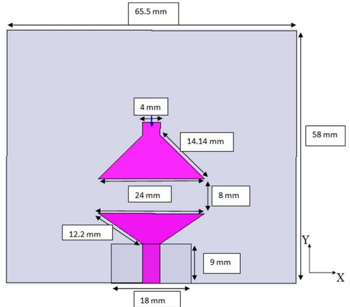
Fig. 5. The “reconfigurable communicating” antenna structure.
