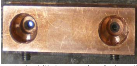
Figure 4: The drilled copper piece for laser diode integration
